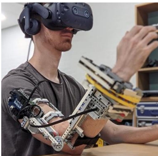
Figure 4. Exoskeleton with Lego pieces and computer interface [5]
